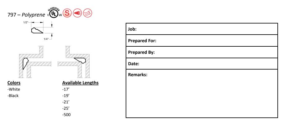
Note: Must be applied on clean, dry frames between 50°F and 100°F. Smoke seals have a pre-installation shelf life of 6 to 9 months.
